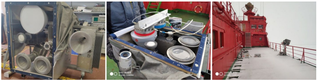
Fig. 8. The complete set of the microwave radiometric complex (a), the complex during calibration using standard emitters (“cold” and “hot” loads) (b), and the complex fixed on board the “Yamal” icebreaker during measurements (c)
