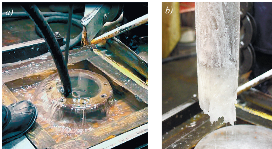
Fig. 4. Overflow of drilling fluid from the borehole mouth during the first unsealing of Lake Vostok (a), and the drill bit covered with frozen lake water after removing the drill from the hole (b)
