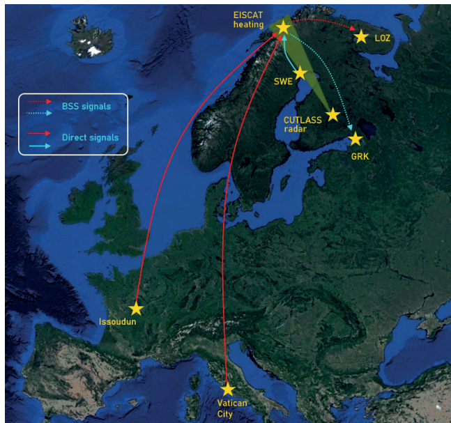
Fig. 1. The geometry of the experiment on 18 February 2013 with the use of the EISCAT HF heating facility, the CUTLASS HF coherent radar, an oblique sounder on the Sweden — Tromsø — St. Petersburg radio path and AM HF broadcasting stations with receivers at GRK and LOZ stations
